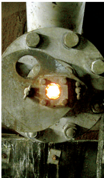
Burn out: a plasma torch gasifies municipal waste, which is used to power a steam turbine at Utashinai.
