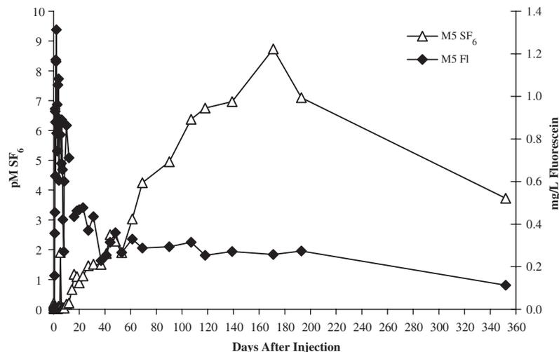
**Fig. 5 – Sulfur hexafluoride (open symbols) and fluorescein (closed symbols) data for well M5 during the Magnolia tracer study. The drainfield was injected on May 24, 2003. The highest concentrations observed in this well were 1.31 mg/L fluorescein at 2.19 days and 8.74 pM sulfur hexafluoride at 171 days after injection.**
