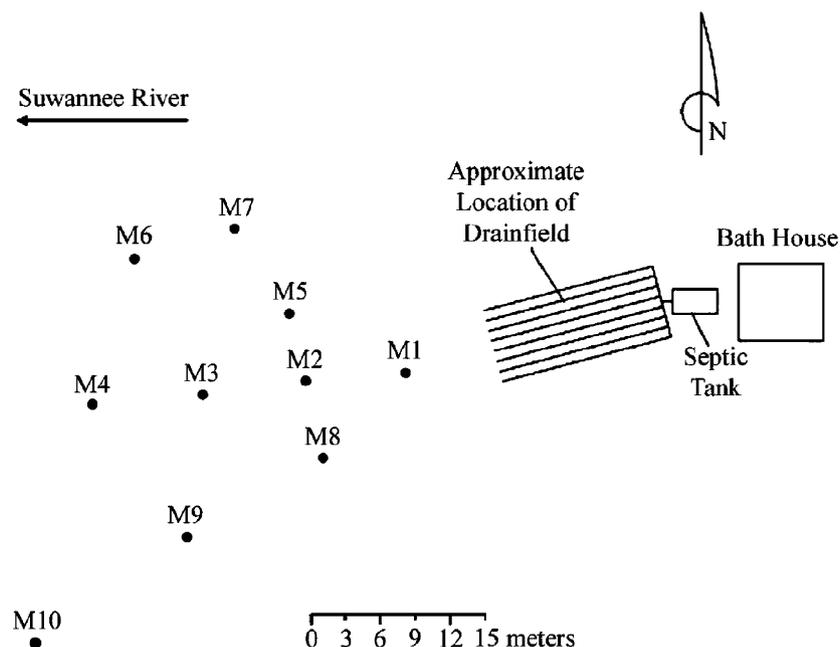
**Fig. 2 – Magnolia site behind the Magnolia II campground bathhouse. Well M1 is in the lower portion of the drain mound slope. Wells M10, M4, and M6 are just in front of the cypress swamp adjacent to the Suwannee River. Groundwater flows towards the Suwannee River in a westerly direction. The order of fluorescein appearance in the wells was M8, M9, M5, M6, M3, M4, M7, M1, M2, M10.**
