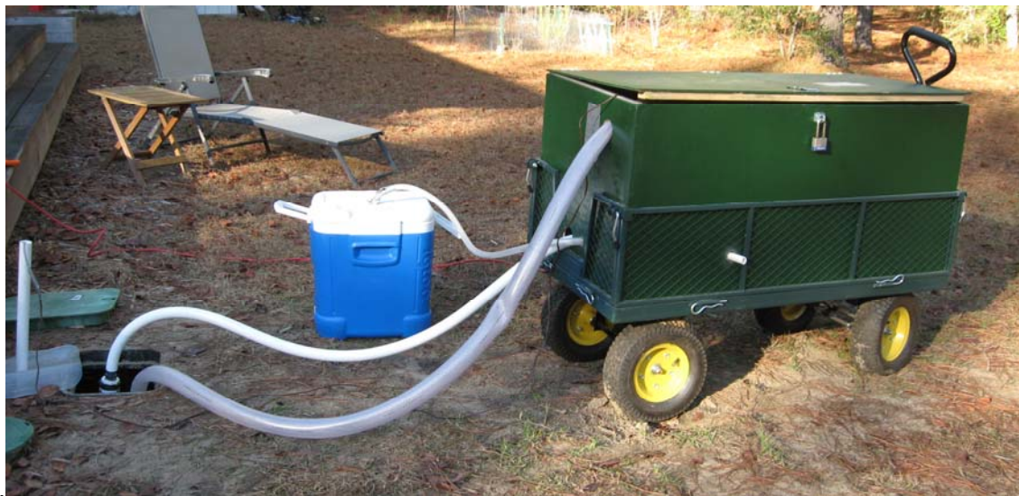
Figure 8. The sampling pump wagon set-up at a residence to sample raw sewage. The clear hose is the inlet to the pump and the white hose is the return line. The blue cooler holds a glass 2 gallon jar on ice. On the far right, the wire coming out of the PVC pipe is from the water sensor.
